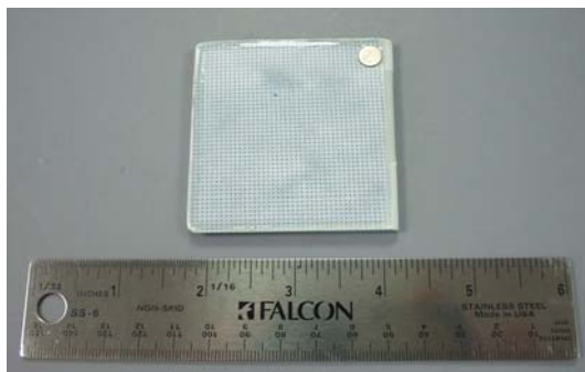
Figure 5: 4 th Generation Zinc-Air Cell
