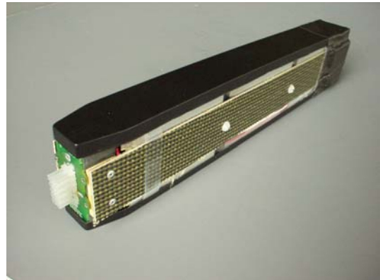
Figure 9: Gen 4 Zinc-Air Dragon Eye Battery
