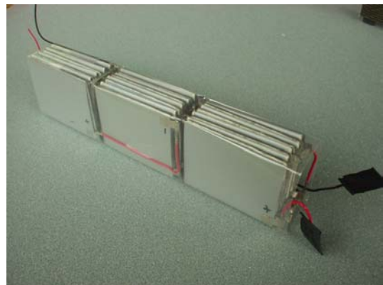
Figure 10: Dragon Eye Battery, Cell Stack Arrangement
